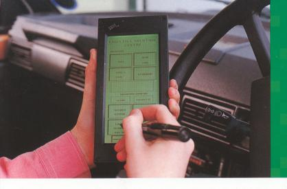
The IBM TouchMobile System is a rugged, touch-screen computer combining a bar-code scanner with on-screen signature and data capture. TouchMobile Solutions provide mobile workers with a flexible, picture driven tool that helps them to work more effectively while improving the use of assets and customer service.
